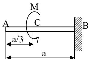
Rješenje:  $r=21,98 \text{ mm}$ ,  $\varphi_A=\varphi_C=0,023 \text{ rad (}1,32^\circ\text{)}$ .
