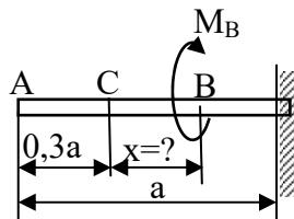
Rješenje:  $x=103,5 \text{ mm}$ ,  $\varphi_A=\varphi_B=\varphi_C$ .
