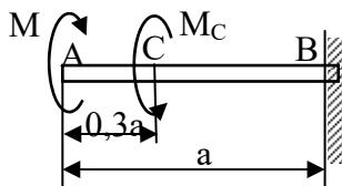
Rješenje:  $\varphi_A=0,08225 \text{ rad } (4,71^\circ)$ ,  $\varphi_C=0,05382 \text{ rad } (3,08^\circ)$ ,  $M=M_C=170 \text{ Nm } (\varphi_C=0)$ .
