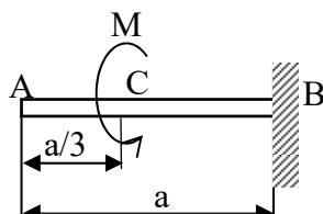
Rješenje:  $\varphi_A=0,015 \text{ rad (}0,9^\circ\text{)}$ ,  $\varphi_A=0,0225 \text{ rad (}1,3^\circ\text{) (M u točki A)}$ .
