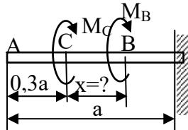
Rješenje:  $x=31,1 \text{ mm}$ ,  $\varphi_C=\varphi_A$ ,  $\varphi_B=0,0134 \text{ rad (}0,769^\circ\text{)}$
