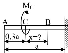
Rješenje:  $x=103,3 \text{ mm}$ ,  $\varphi_A=\varphi_C=0,01086 \text{ rad (}0,622^\circ\text{)}$ ,  $\tau_{A-C}=0$ ,  $\tau_{C-B}=19,1 \text{ MPa}$ .
