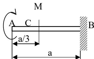
Rješenje:  $M=125,7 \text{ Nm}$ ,  $\varphi_A=0,060 \text{ rad (}3,44^\circ\text{)}$ ,  $\varphi_C=0,045 \text{ rad (}2,29^\circ\text{)}$ .
