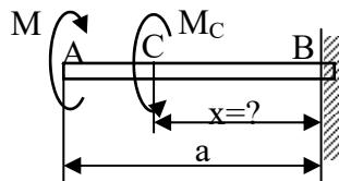
Rješenje:  $x=513,3 \text{ mm}$ ,  $\varphi_C=0,0153 \text{ rad (}0,878^\circ\text{)}$ .
