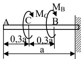
Rješenje:  $M_B=33,94 \text{ Nm}$ ,  $\varphi_B=0,00859 \text{ rad (}0,492^\circ\text{)}$ .
