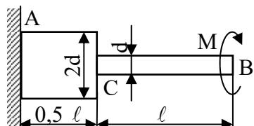
Rješenje:  $M=0,457 \text{ Nm}$ ,  $\varphi_C=0,0000909 \text{ rad (}0,0052^\circ\text{)}$ .
